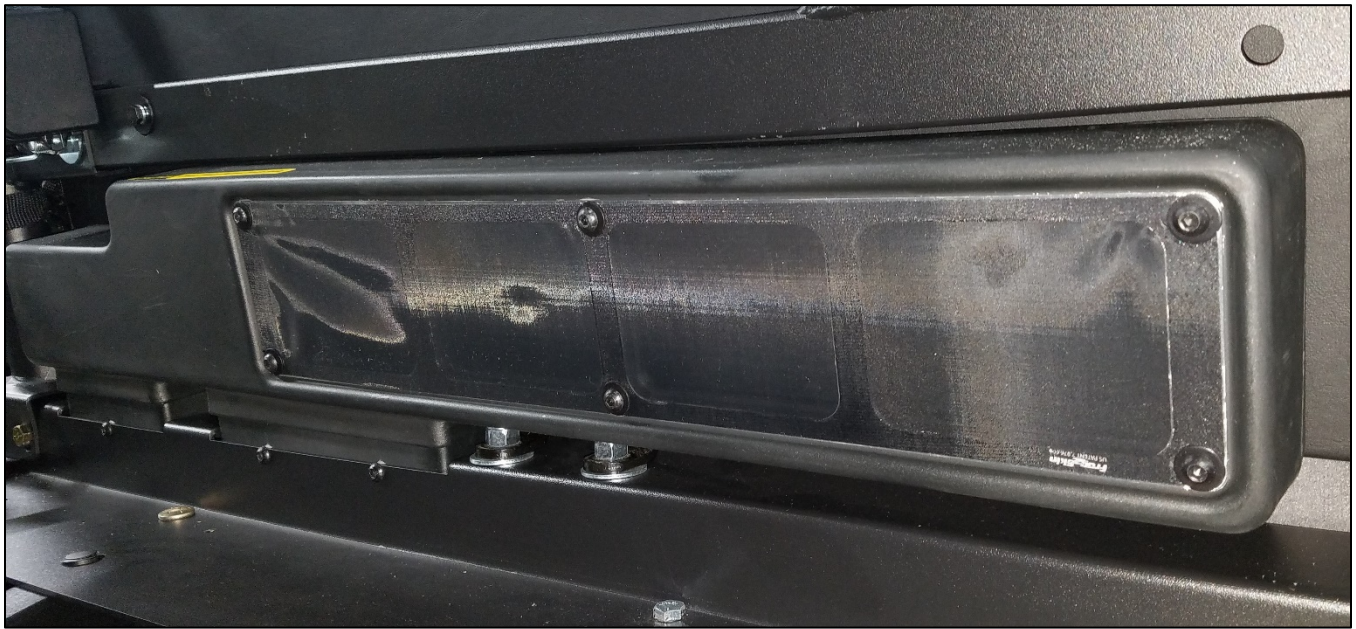
Figure 21: Air Intake Screen
